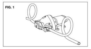
Note: To help reduce noise and vibration of the pump through the system use flexible lines on the inlet and outlet of the pump as shown above. Be sure to use lines rated to not collapse under pump vacuum.
